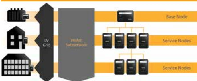
**Fig 2: Main Components of a PRIME Sub-Network**
