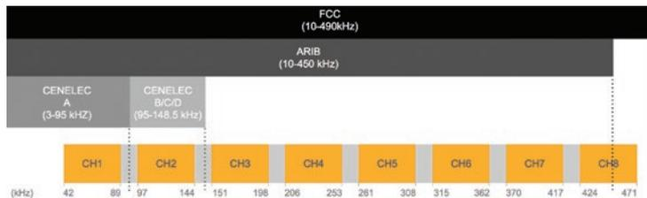
PRIME specifications now support frequency ranges going from the CENELEC A-band (<95kHz) up to 500 kHz, allowing for optimum usage in electric grids all over the world. Robust transmission modes have been designed to improve system performance against both high power impulsive noise and interfering noise. PRIME can be fitted for multiple
